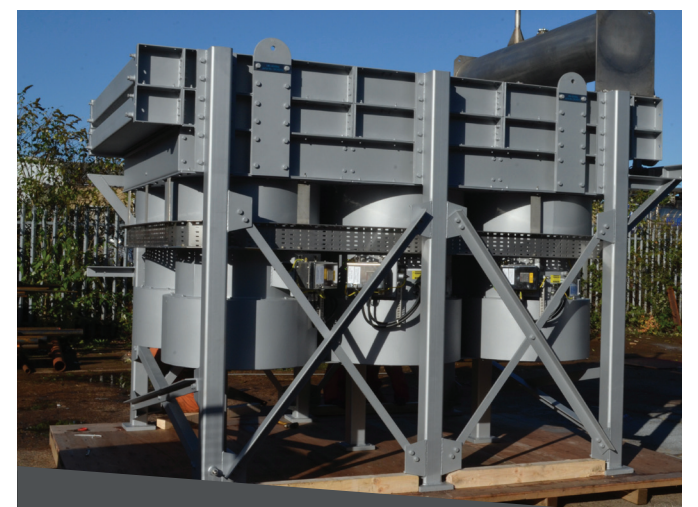
Remote radiator for MTU 16V4000, offshore generator set
